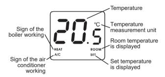
This wireless (radio-frequency) thermostat can also be easily extended with the **COMPUTHERM Q1RX** socket if needed, with which the thermostat is able to control boilers or any other electrical devices operating on 230V (50Hz; max. 16A) (e.g. fan heaters, pumps, zone valves, etc.) according to the room temperature. (You can find detailed information and recommended usage of the **COMPUTHERM Q1RX** socket on our website: www.quantrax.hu)
