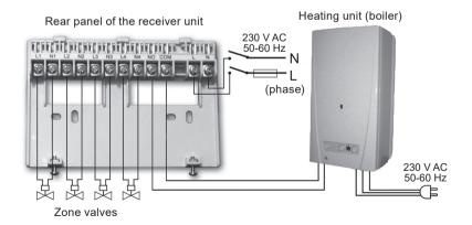
Cut or break out the outlets to the required connection points at the bottom of the receiver unit, in order to be able to connect wires to them.
