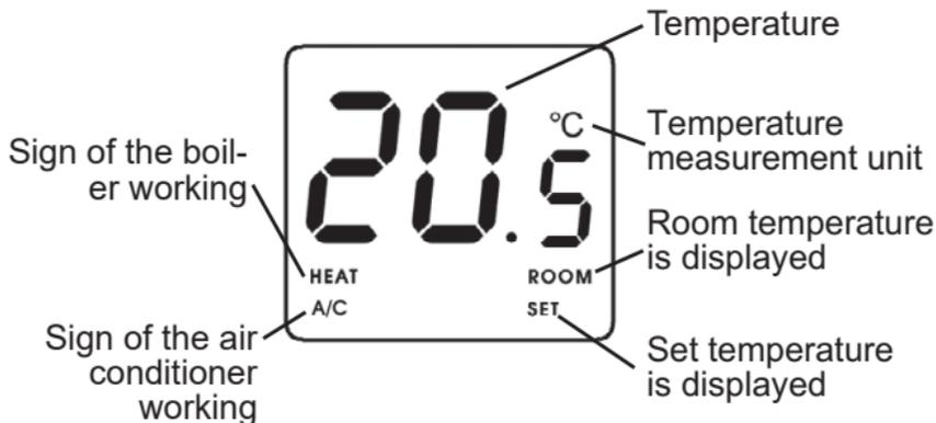
The device consists of two units. One of them is the portable control unit (thermostat), while the other unit is the receiver that controls the boiler. Because there is a wireless (radio-frequency) connection between the two units, no cable is required between the thermostat and the boiler. The two units have been tuned in the factory so that they operate at the same
