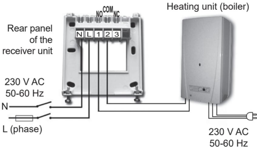
If you would like to operate an old boiler or any other device that has no connection points for thermostats, then the **No. 1** (NO) and **No. 2** (COM) connection points of the thermostat should be connected to the mains cable of the device, similarly as a switch would be connected.
