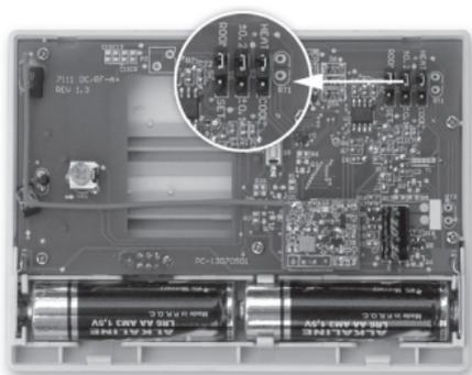
After the batteries have been inserted, the display flashes the measured room temperature. (If this information fails to appear on the display, press the „**RESET**” button located on the main panel of the thermostat.
