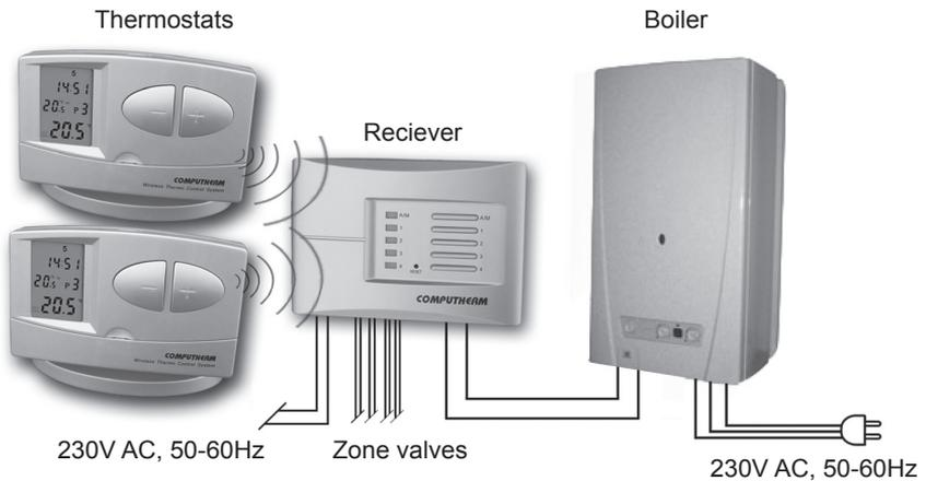
The device can be programmed according to customer-specific requirements so that the heating/cooling system heats/cooling your residence or office to the required temperature at the dates and times specified by you, to reduce energy costs while maintaining comfort. Separate temperature programs can be prepared for each day of the week. For each day, beside 1 fixed switching time, 6 adjustable switching times can be set and a different temperature can be assigned to all 7 switching times.
