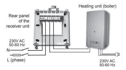
Unscrew the two screws at the bottom of the receiver unit without removing them. Following this, remove the front panel of the receiver unit then fix the back panel to the wall in the vicinity of the boiler with the screws provided. Remove the protective carton from the contacts to ensure perfect contact.
