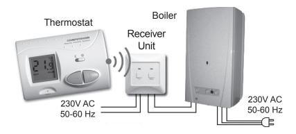
The effective range of the transmitter incorporated in the thermostat is approximately 50m in open terrain. This distance may become considerably shorter within a building, especially when a metal structure, reinforced concrete or adobe wall stands in the way of radio waves.
