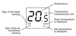
The device consists of two units. One of them is the portable control unit (thermostat), while the other unit is the receiver that controls the boiler. Because there is a wireless (radiofrequency) connection between the two units, no cable is required between the thermostat and the boiler. The two units have been tuned in the factory. The trouble-free operation is ensured by its own security code. The installation and connection of the receiver unit is described in **Chapter 7**.
