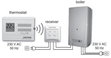
Temperature can be measured and set more precisely as compared to simple, conventional thermostats. In heating mode, in accordance with the selected switching sensitivity, the thermostat switches the boiler or any other appliances on and off below and above the adjusted temperature, respectively, and contributes to reduce energy costs while maintaining comfort. In cooling mode it switches exactly the opposite way.
